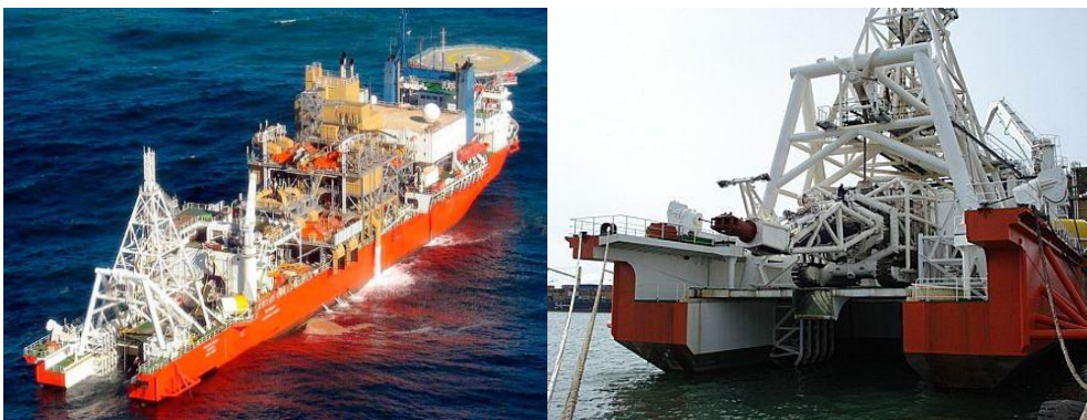
Fig. 4 Offshore diamonds mining vessel (left) and the subsea crawler (right)
